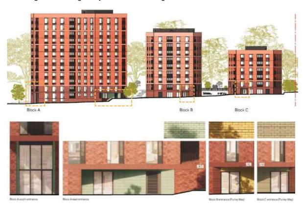
Image 8: Purley Way Elevation detailing the proposed principle tonality across the site (top) and proposed main entrances (bottom)
